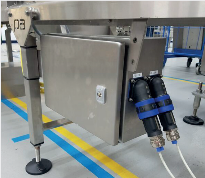
Han® F+B in action, configured as hood with angled bulkhead mounted housing
